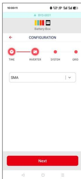
Figure 11 Inverter Configuration
