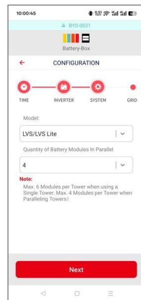
Figure 12 System Configuration
